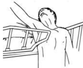
Entrapment between split bed rails
