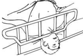
Entrapment under the bed rail
