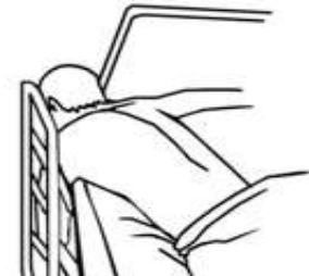
Entrapment between the end of the rail and the side edge of the headboard or foot board
